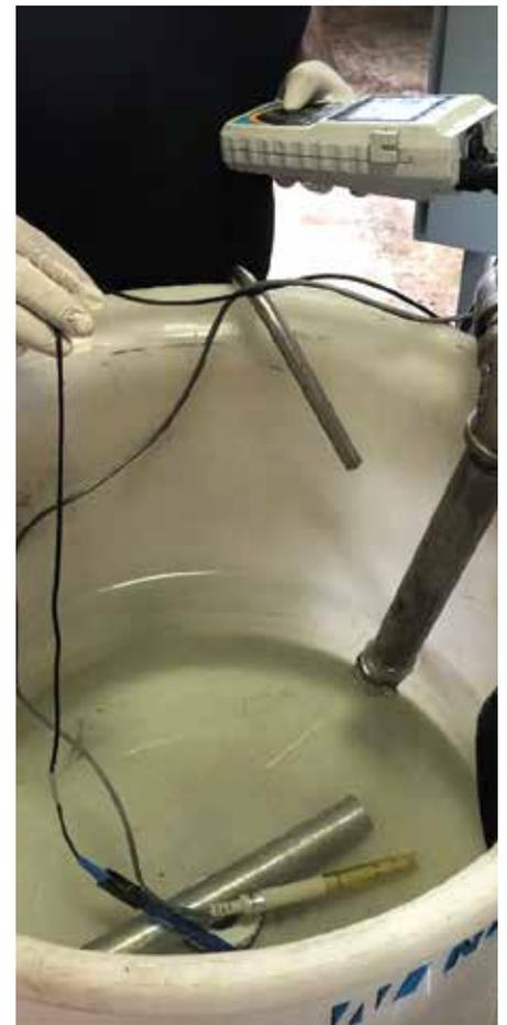
Figure 5. Measuring the conductivity of the permeate (clear water)
